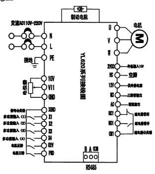
制动电阻: Braking resistor (+DB-)
