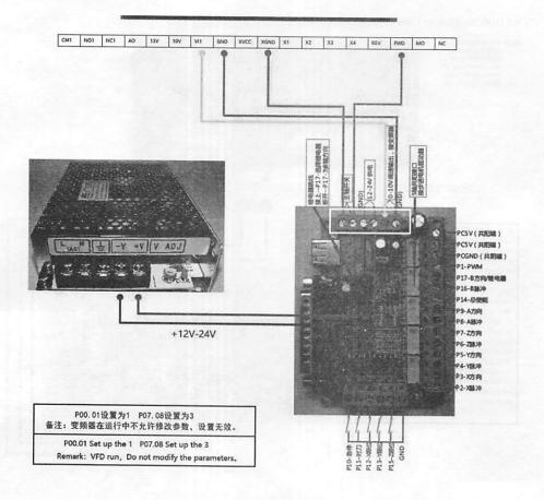
6.5 External potentiometer with switch control wiring and parameter setting:
