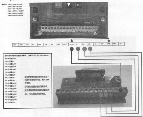
6.4 Analog quantity control wiring and parameter setting:
