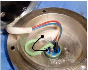
inside. Solder the other end of wire to pin 4 solder lug of the plug; using wire at least the same gauge as your spindle cable.
